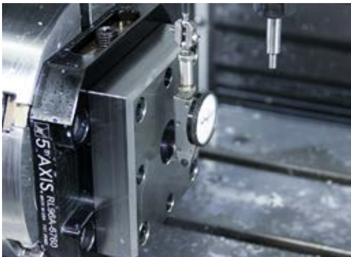
Precision center bore allows for indication of rotation.
