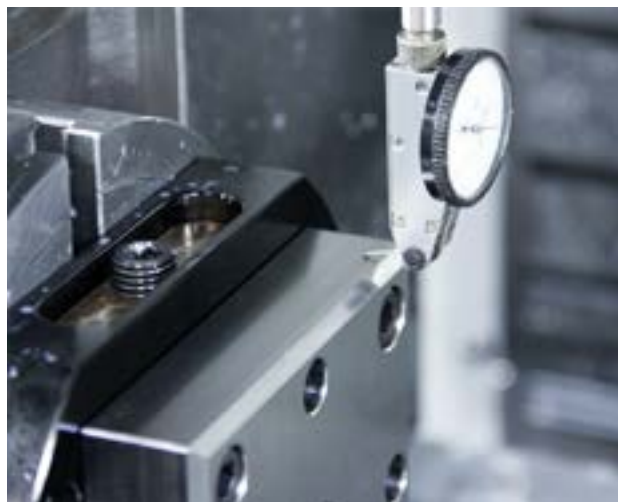
Precision milled sides allow for indication of center line.
