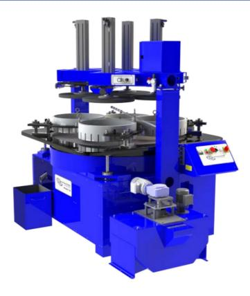
The Lapmaster Model 56 is equipped with a 56 inch (1422mm) diameter lap plate. This is manufactured from Grade 300 grey cast iron to ISO 185(2005). It consists of individual segments bolted to a support plate.
