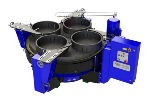
The Lapmaster Model 72 is equipped with a 1829mm diameter lap plate. This is manufactured from Grade 300 grey cast iron to ISO 185(2005). It consists of individual segments bolted to a support plate.
