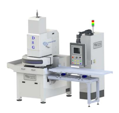
The Lapmaster DSG range of dual face fine grinding machines is based on a three way planetary concept, designed to yield precise and repeatable results at an economical price. Excellent results are obtained in the processing of a wide range of materials and components including glass, ceramics, crystals and ferrous metals.
