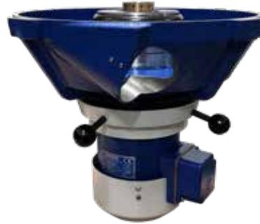
All the spindles are equipped with the Coborn Expanding Nose System as standard, which has removed the problems of mounting and dismantling scaife plates where there is a tight fit on the spindle nose. The expanding nose also improves the quality of polish especially if the scaife plate has an oversize bore on a parallel nose, which may result in the scaife plate taking a random position causing unbalance and vibration.
