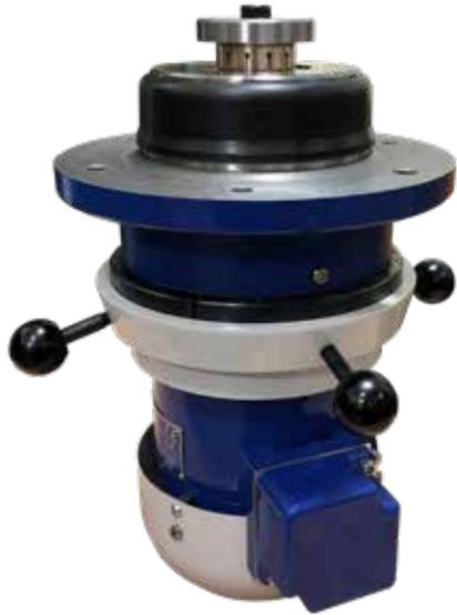
Without an inverter, these 3 phase spindles may be directly wired to run at 2,860 rpm at 50Hz (or 3400rpm at 60Hz). An inverter can also be fitted to give speed control from 1,500 rpm -- 4,200 rpm.
